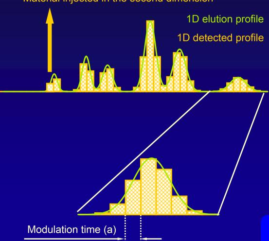
Second-dimension separation operates as the detector for the first dimension
